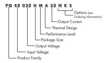
The first 12 characters comprise the base part number and the last 3 characters indicate available options. Although there are no default values for enable logic and pin length, the most common options are negative logic and 0.145" pins. These part numbers are more likely to be readily available in stock for evaluation and prototype quantities.
