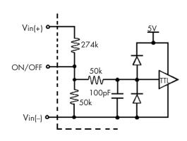
Figure B: Internal ON/OFF pin circuitry
